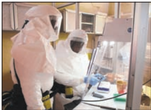
WORKING ON A CURE: A technician sets up an assay for Ebola within a containment lab. Samples are handled in negative-pressure biological safety cabinets to provide an additional layer of protection.
