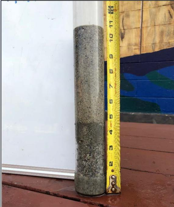
**Confirmation Cores** were taken prior to catch pan retrieval as an initial check of cap layer thickness.
